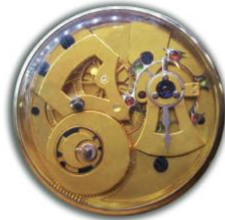
Sand-blasted gilded main and top plates (Watch Museum of Le Locle collection) (MHL collection)
