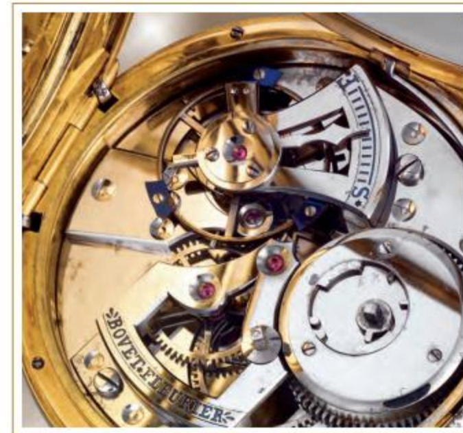
Polished steel main and top plates (Bovet private collection)
