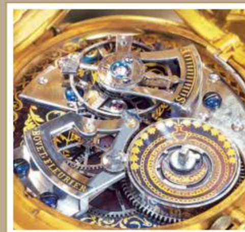
Mainplate and certain top plates in polished blued-steel (photo provided by Antiquorum)
