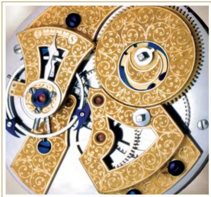
Polished steel mainplate and gilded brass top plates engraved with decorative pattern (private collection)
