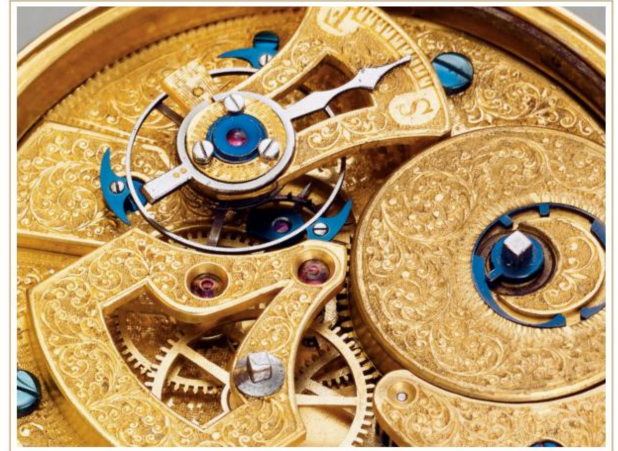
Gilded brass main and top plates engraved with decorative pattern, eight-day power reserve and two train wheel bridges (Pascal Raffy private collection)
