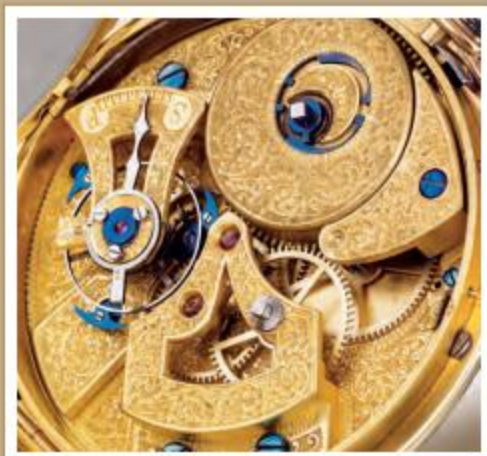
Brass main and top plates engraved with decorative pattern, eight-day power reserve and two train wheel bridges (Pascal Raffy private collection)
